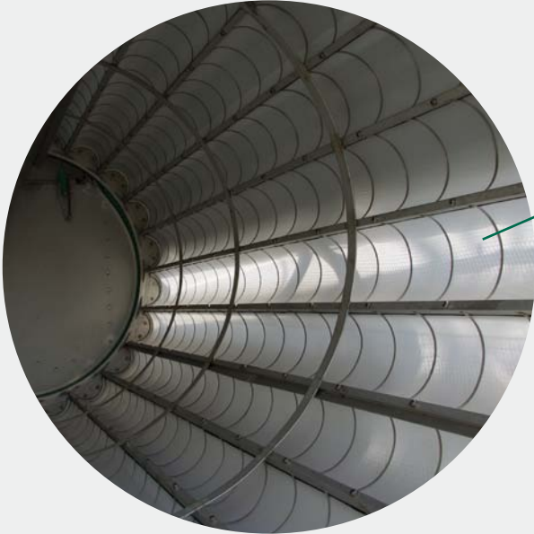
The micro drum with filter cloth segments and discharge hopper of reject
